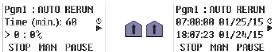
When this screen first appears, the sample containers should be replaced with empties.
