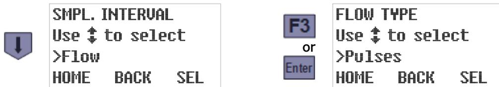
Use the Up or Down key to scroll to the desired type, then press the SEL [F3] or Enter key to save it and display its first setting:
