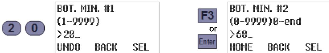
The digit keys can then be used to change the number of minutes the program would wait between samples for the second bottle. Pressing the SEL [F3] or Enter key would again save the displayed value and display the next. And so on until pressing the SEL [F3] or Enter key while Bottle Minutes #24 is displayed restores the Program Configuration menu scrolled to its next group (Bottle Options).
