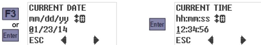
The same techniques are used to change both settings. The third line displays the current value, with an underline cursor indicating the digit currently subject to editing:
