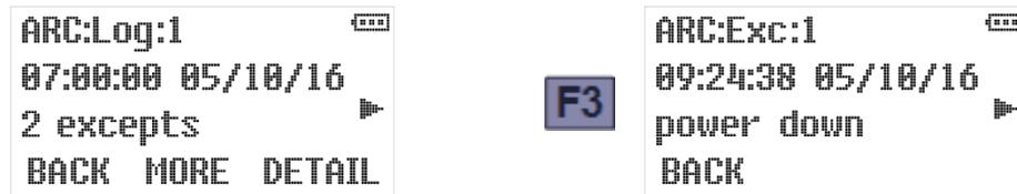
where the screen shown to the left indicates that the program run that commenced at 7:00 AM on May 10 encountered two exceptions. The screen on the right indicates the first of them was an electrical power loss at about 9:25 AM on that same date.
