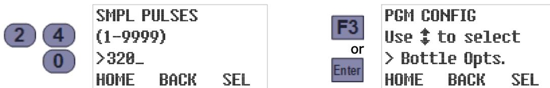
You can repurpose the flow-pulse input to initiate a sample each time a connected PLC or other external device closes its circuit (see page 88). In that case, you would of course set this parameter to 1.
